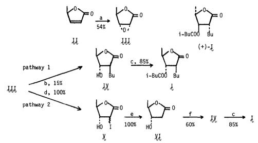
a: NaOCl, pyr. rt; b: Bu<sub>2</sub>CuLi, ether, -20°; c: i-BuCOCl, pyr, rt; d: NaI, NaOAc, AcOH, acetone; e: H<sub>2</sub>, Pd/C, EtOAc; f: i) LDA, THF, -78°, ii) BuI, HMPA, -40°, yield based on transformed starting<sup>2</sup>material.
